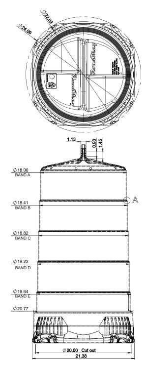
MATERIAL:IMPACT-RESISTANT POLYETHYLENE COLOR:UV-STABILIZED HIGHWAY ORANGE
