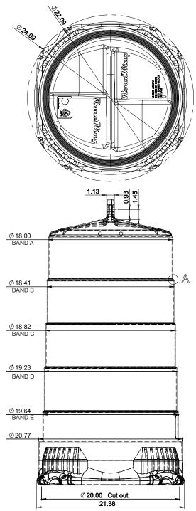
MATERIAL:IMPACT-RESISTANT POLYETHYLENE COLOR:UV-STABILIZED HIGHWAY ORANGE
